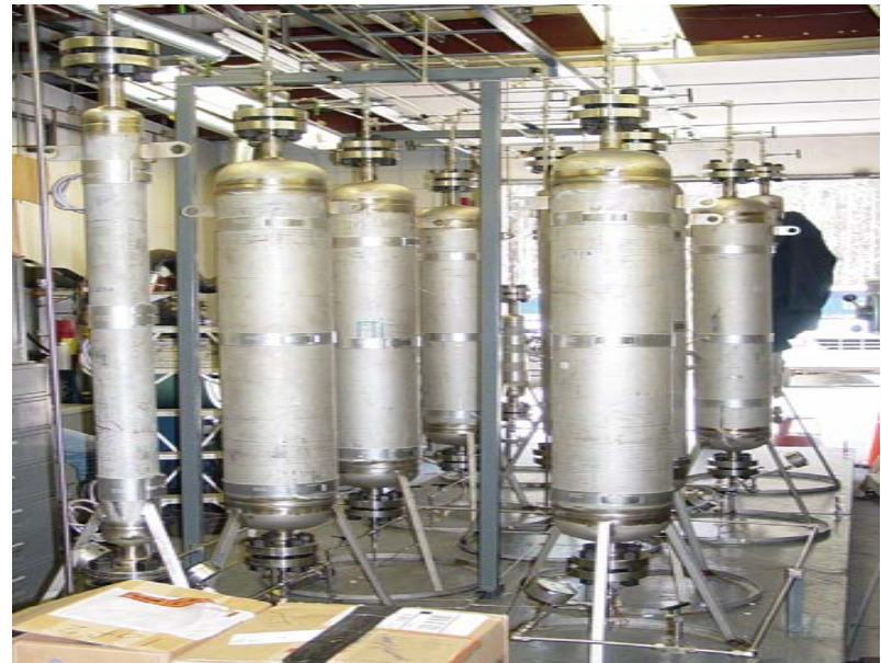
Ammonia and trace metal skid for testing at Eastman
